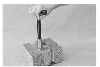
Figure 7. Removing the Vapor Pin<sup>™</sup>.
