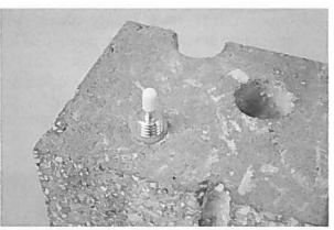
Figure 4. Installed Vapor Pin<sup>TM</sup>.
