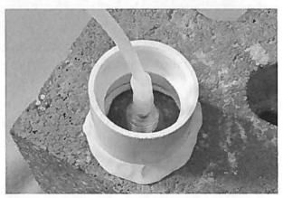
Figure 6. Water dam used for leak detection.
