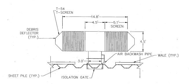
Figure 4-5 Cylindrical Wedge Wire – Typical Section
