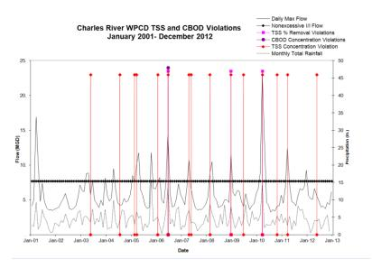
Figure 7. CRPCD CBOD and TSS Effluent Limit Violations
