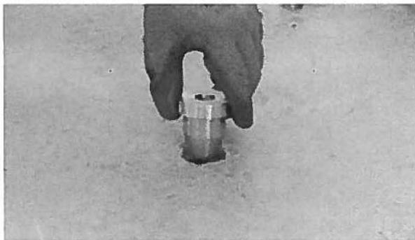
**Figure 3.** Installing the Drilling Guide.
