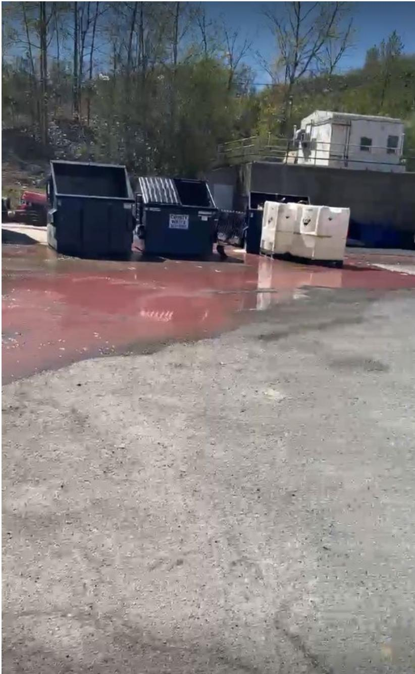
4. From Video IMG\_1300 – May 9, 2022, Untreated process wastewater from EQ tank overflowing flowing towards storm drain/catch basin.
