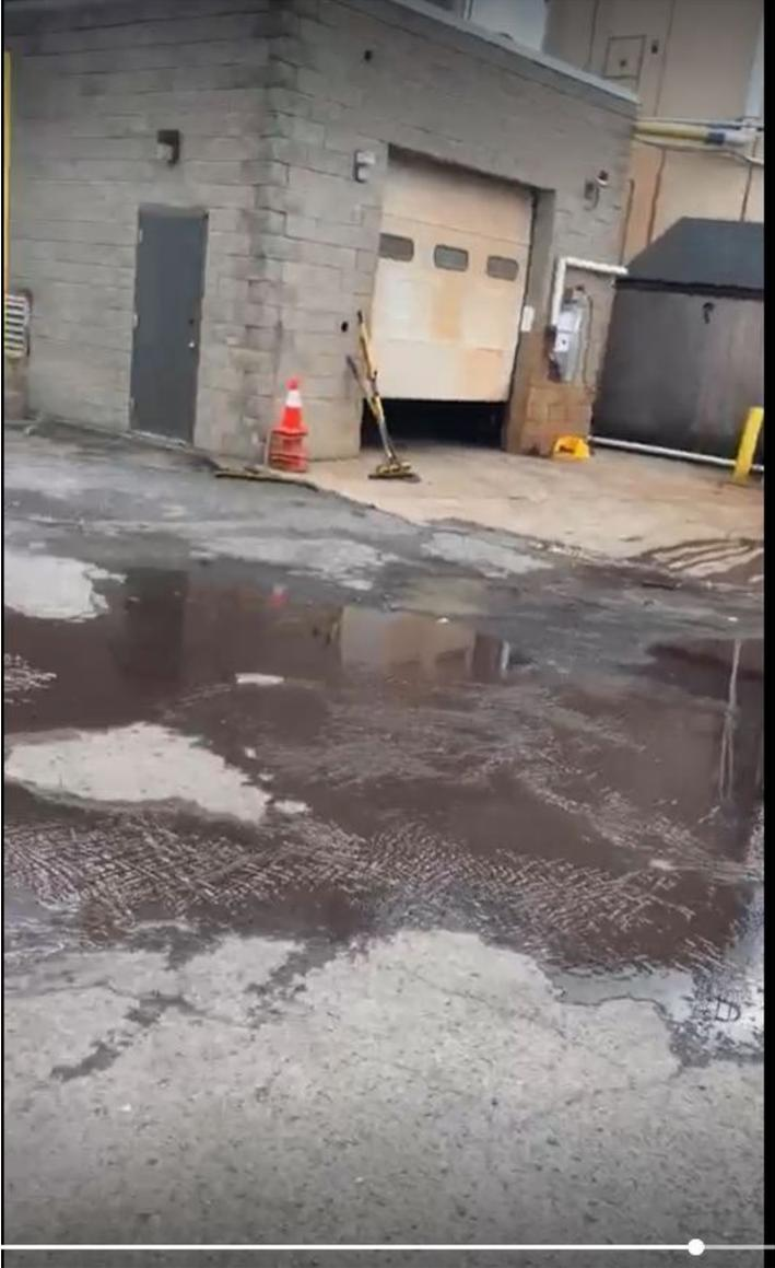
4. Wet well overflow wastewater flowing towards storm drain
